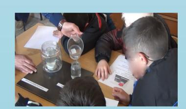
Both glass jars were filled with hot water. The initial temperature of the water was measured with an infrared speaking thermometer and recorded by the students and then lids of the jars were closed.
